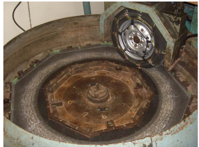
Fig. 3. The apparatus of surface abrasion test (“raveling test” method based on Japanese standard pavement tests (Hosoubinran 3-7-2)).
